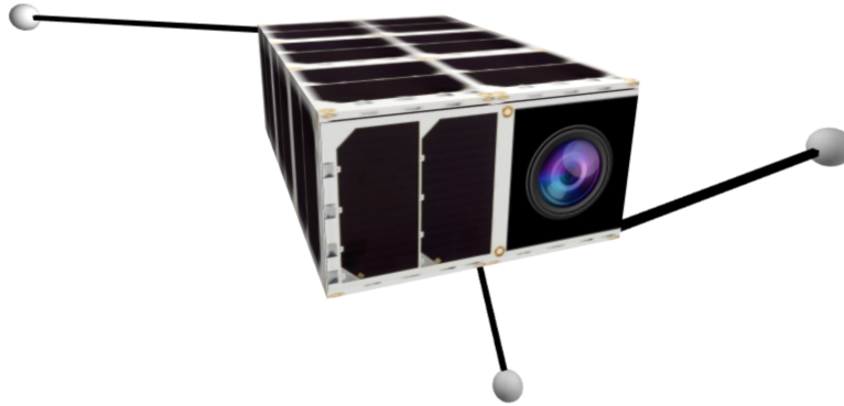
Figure 6.1: Proposed architecture for a 6U CubeSat space telescope. Each boom has a single degree-of-freedom in linearly independent axes, enabling three-axis attitude control. Magnetorquers are used to desaturate the angular momentum of the booms and keep them within their operating limits.
